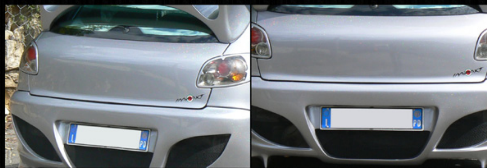
LTPE0101 - Lisciatura baule in vetroresina | Smoothing trunk
